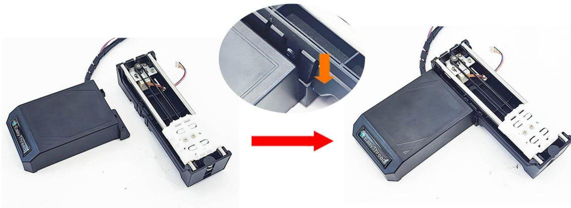
2, assemble with the Y-axis and snap the Y-axis into the white snap position on the X-axis.
