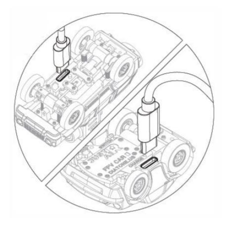
Light flashing: Normal charging. Lights off: Charging complete.
