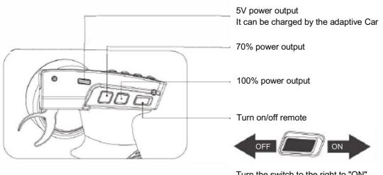
Turn the switch to the right to "ON". Turn on the power of AIR 5, you can enter the working state.
